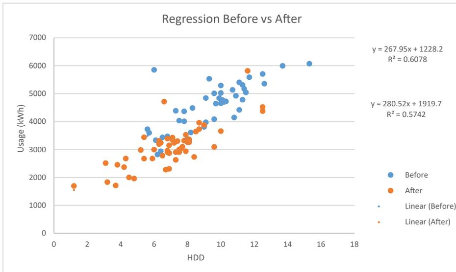
Due to the availability of half hourly data, the analysis of EndoTherm was undertaken using the IPMVP methodology for comparing energy saving trials. A regression analysis for both data sets was taken and trend-lines drawn for each time period.
